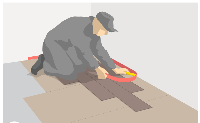
6 Perimeter insulation barrier cut
