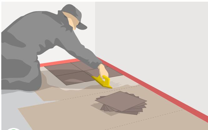
3 Final floor application (glued)
