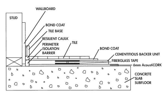
Tile Floors over 1/2" CBU's on a Concrete Slab
